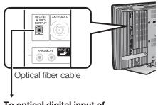
To optical digital input of external audio devices
